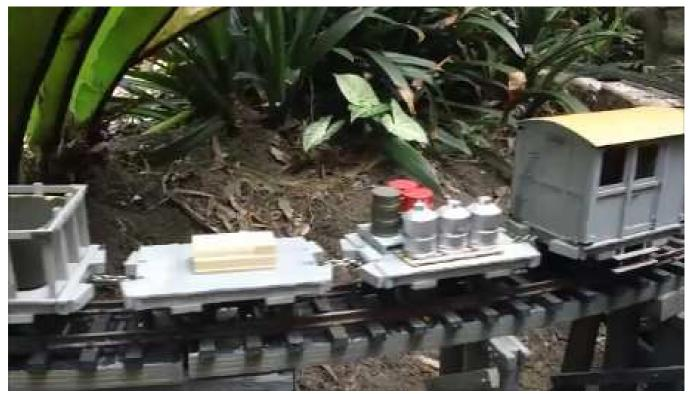
These Flat Wagons are scratch built of wood, the wheels are 25mm diameter Bachmann brand.
